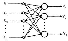
Fig. 2. Forward propagation neural network
